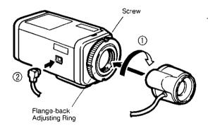
When using a lens other than those listed on pages 9, 10, 11, 12 and 13, the lens mount should be C-mount or CS-mount (1\*-32UN) and the lens weight should be less than 0.99 lbs. (450g). If not, both the lens and camera should be supported.
