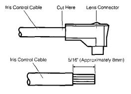
(2) Remove the insulation of the individual iris control wires as shown in the diagram below.
